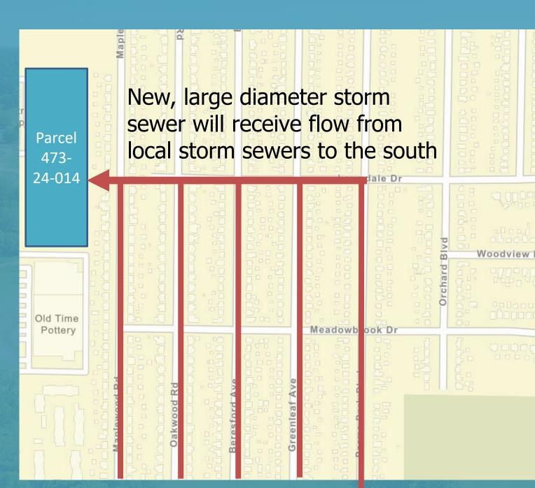
Next steps to relieve flooding: **Stormwater and Sanitary Sewer Work** • Coordinate with City on phasing and funding of infrastructure planning and design Sanitary sewer system in this area of Parma Heights was a focus of LSSES; strong candidate for a District grant through the Member Community Infrastructure Program
